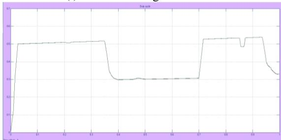
**Fig. 5 Change in Duty Cycle of P & O MPPT Algorithm**
