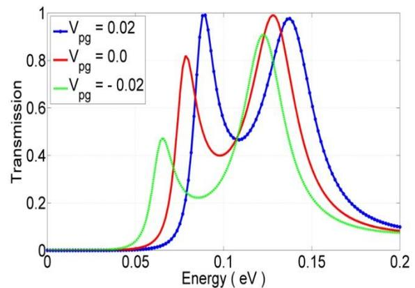
**Figure 3. Transmittance versus electron energy of the negative bias voltage  $V_{bias} = 0.16$  eV for three different value of  $V_{pg}$ ,  $V_{pg} = 0.02$  V (blue dotted line),  $V_{pg} = 0.0$  V (red line) and  $V_{pg} = -0.02$  V (green dotted). The TB-lead coupling  $t = 0.175$  eV, and  $\mu_L - \mu_R = eV$ . Length of each quantum well is 2.7nm, the barrier width  $W_b = 0.3$  nm.**
