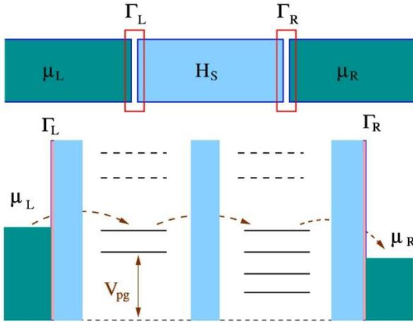
**Figure 1. Schematic representation: of the central system and the two leads (top panel), and the energy levels of the TB system with broadening coupling  $\Gamma_{L,R}$  in the transfer region (bottom panel) in the case of positive bias. The chemical potential of the left and the right leads are denoted as  $\mu_L$  and  $\mu_R$  respectively.**
