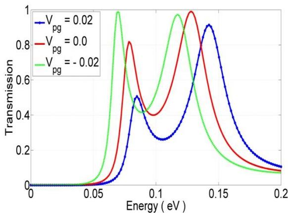
**Figure 2. Transmittance versus electron energy of the positive bias voltage  $V_{bias} = 0.16$  eV for three different value of  $V_{pg}$ ,  $V_{pg} = 0.02$  V (blue dotted line),  $V_{pg} = 0.0$  V (red line) and  $V_{pg} = -0.02$  V (green dotted). The TB-lead coupling  $t = 0.175$  eV. Length of each quantum well is 2.7nm, the barrier width  $W_b = 0.3$  nm.**
