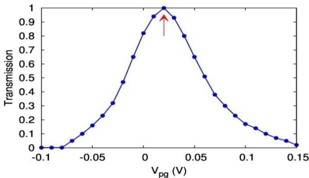
**Figure 4. Transmittance versus plunger-gate voltage for the case of  $V_{pg} = 0.02$  of the Fig. 3 (blue dotted line). Electron energy  $E = 0.08$  eV,  $t = 0.175$  eV. The other parameters are the same as Fig. 3.**
