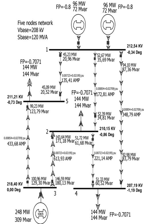
**Fig. 13. One line diagram of five nodes network for base case (Power World solution).**
