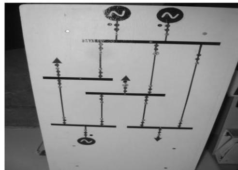
**Fig. 11. Physical simulator to load flow studies, developed at UAEM**
