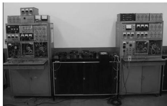
**Fig. 12. Complete physical simulator to load flow and voltage stability**
