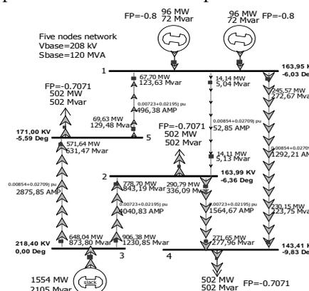
**Fig. 18. One line diagram of five nodes network for tip of the nose case (Power World solution).**
