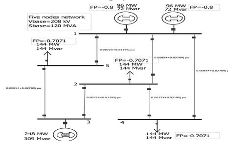
**Fig. 10. One line diagram of five nodes network showing the three phase values for digital calculation**
