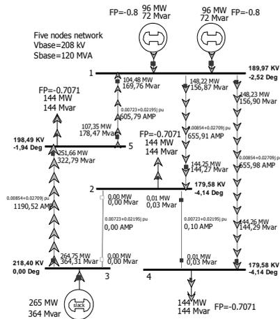
**Fig. 14. One line diagram of five nodes network for contingency case (Power World solution).**
