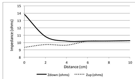
**Fig. 9. Behavior of line impedance versus vertical distance separation.**
