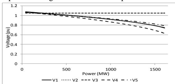
**Fig. 16. P-V curves of the five nodes grid for base case.**
