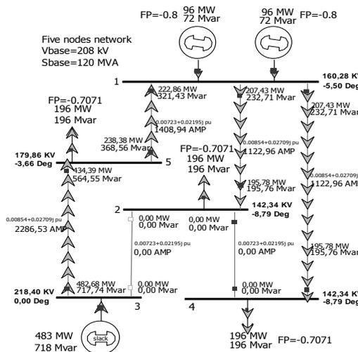
**Fig. 19. One line diagram of five nodes network for tip of the nose contingency case (Power World solution).**
