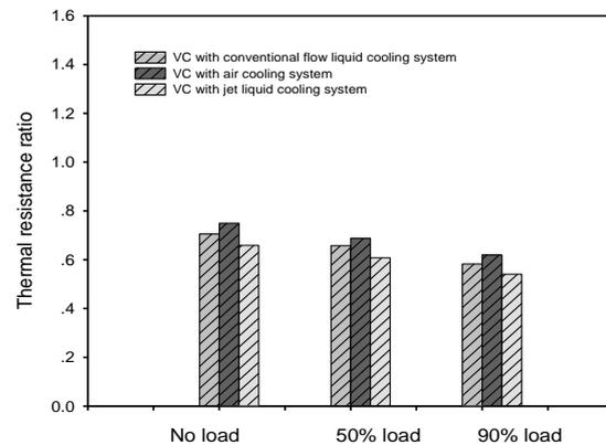
Fig 5 Variations of thermal resistance ratio for different operating conditions of PC
