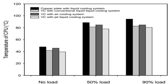
**Fig 3 Variations of CPU temperature for different cooling techniques**
