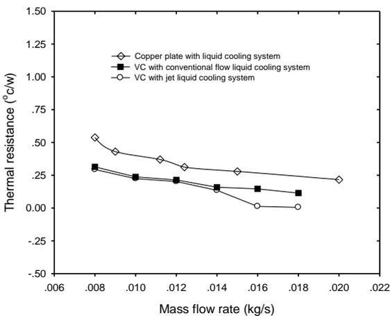
Fig 4 Comparison thermal resistant with mass flow rate for different cooling techniques
