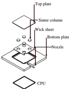
**Fig 2 Schematic diagram of the vapor chamber details**
