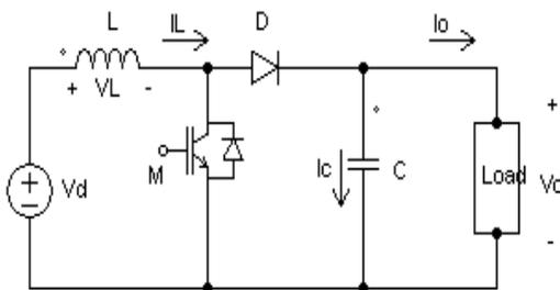
Fig. 3. Circuit diagram of boost converter [8]
