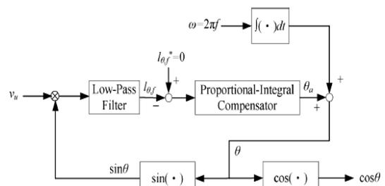
Fig. 7. Digital PLL control scheme [4]
