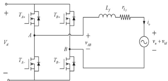
Fig. 5. Grid connected power supply framework [10]
