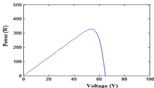
Fig. 8. PV curve of a single PV panel
