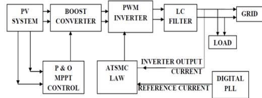
Fig. 1. Block Diagram of Grid Connected PV System
