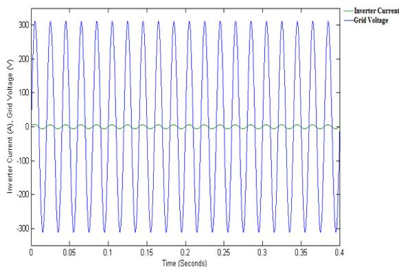
Fig. 12. Synchronization of inverter current with grid voltage
