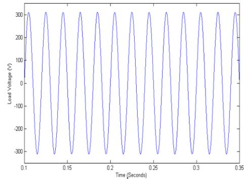
Fig. 13. Load voltage response in grid connected mode
