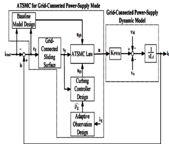
Fig. 6. Block diagram of ATSMC for grid connected power supply mode [4]
