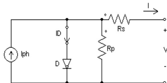
Fig. 2. Equivalent Circuit of a PV cell [8]
