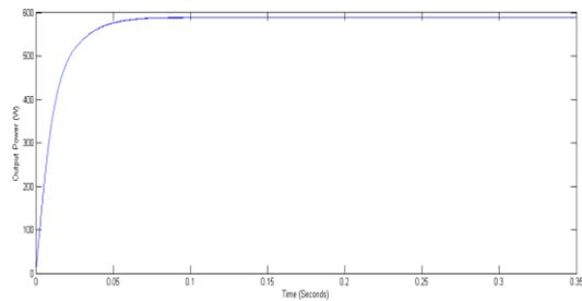
Fig. 9. Output power curve of MPPT controller
