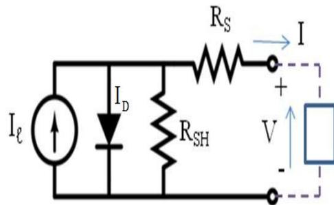
Fig 4: Equivalent circuit of PV Module
