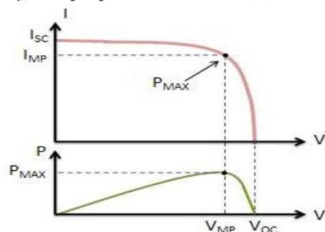
Fig 5: Output characteristics of PV Array
