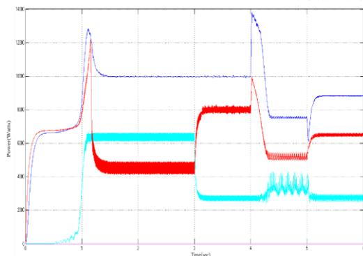
**Fig 10: Both Wind & PV Array without using Battery at a load of 10kW and an Extra load of 4kW**
