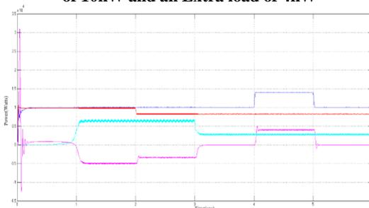
**Fig 11: Both Wind & PV Array by using Battery maintain at a load of 10kW and an Extra load of 4kW**
