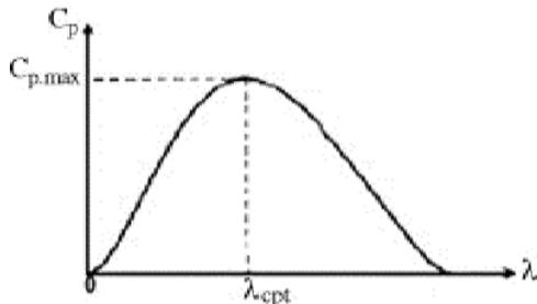
Fig 2: Power coefficient Vs Tip Speed Ratio
