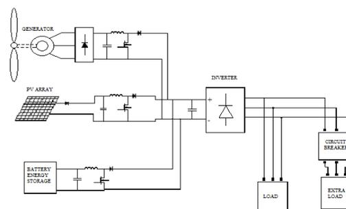
Fig 1: Configuration of Hybrid Energy System
