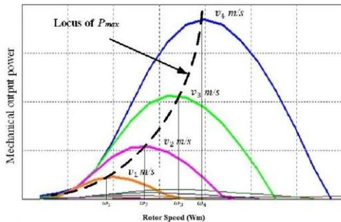
Fig 3: Output Power Vs Rotor Speed of different speeds
