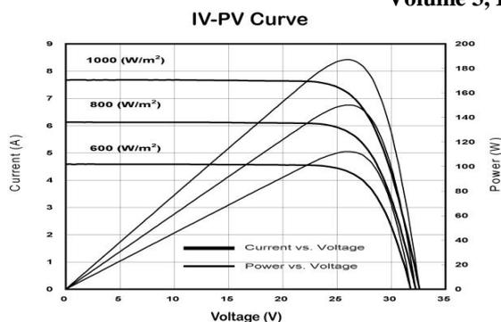
Fig 6: I-V and P-V Characteristics of PV Array at different solar intensities
