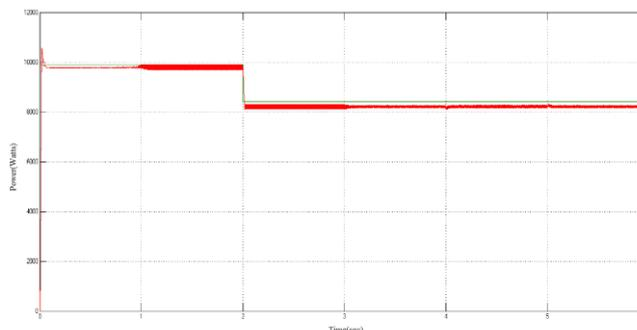
**Fig 8: PV Array Output at different Irradiation levels of 1000W/m<sup>2</sup> and 850W/m<sup>2</sup>**
