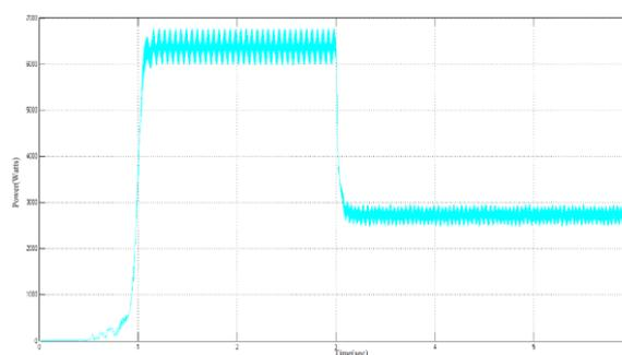
**Fig 7: Wind Power output at a different speed of 12 m/s and 9 m/s**
