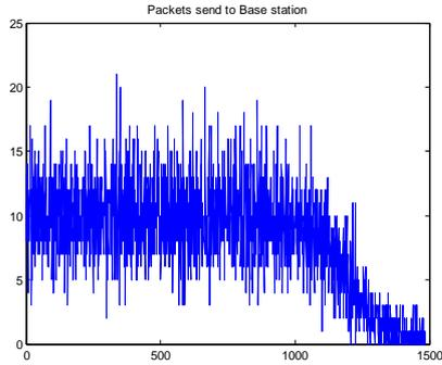
**Fig 6 is Packets that are sent to Base Station in LEACH Protocol.**
