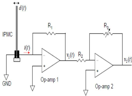
Fig.4. Circuit for measuring the short-circuit current generated by the IPMC sensor.
