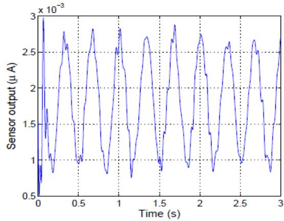
Fig.6. A typical IPMC sensor signal, showing clear periodicity of the source
