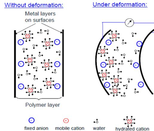
Fig.2. Illustration of IPMC sensing principle.
