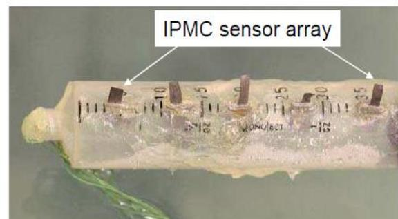
Fig.3. The IPMC-based lateral line prototype
