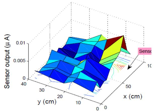
Fig.7. Measured sensor signal amplitude as a function of source location: flapping tail stimulation. The signal was from a single IPMC sensor, the location of which was marked in the figures
