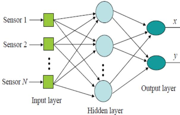
**Fig.8. Schematic of the MLP neural network for signal processing of the IPMC lateral line**
