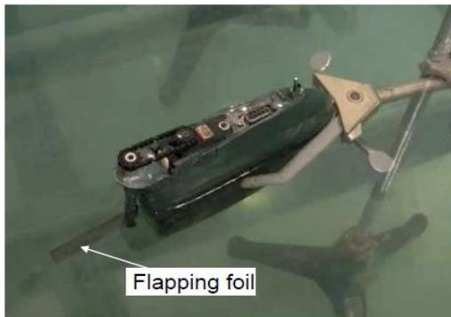
Fig.5 Stimuli sources used for the lateral line sensor: a flapping foil.
