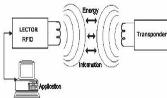
**Fig 1. Schematic of a RFID System**
