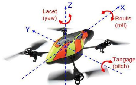
Fig.2. Quadrotor AR.Drone
