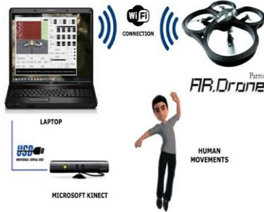
**Fig.3. Principle of connection between the AR.Drone and the Kinect**
