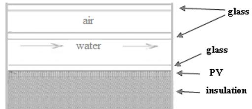
Fig. 2. Descriptive scheme for a solar photovoltaic thermal (PV/T) water collector
