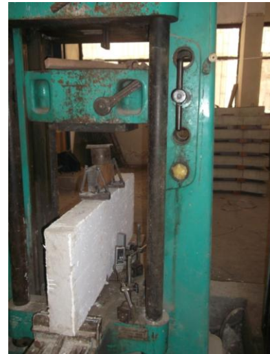
Fig 3. Test setup for deep beams.
