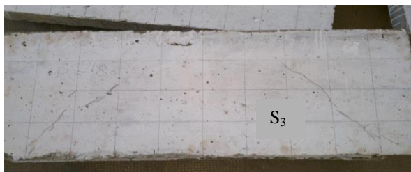
Fig 8. Crack pattern at failure of beams without web opening: (a) V_f = 0\% , (b) V_f = 0.75\% , (c) V_f = 1.0\% .
