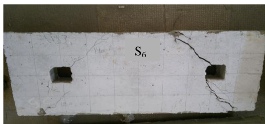
Fig 9. Crack pattern at failure of beams with web opening at 15 cm: (a) V_f = 0\% , (b) V_f = 0.75\% , (c) V_f = 1.0\% .
