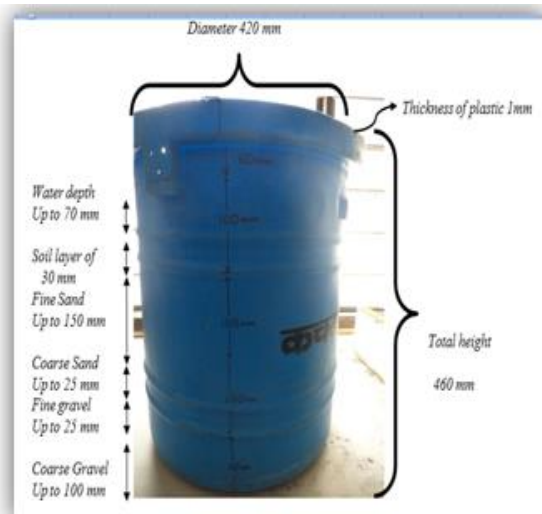
Fig. No.7 Construction of Filter Body
