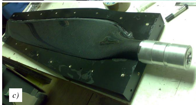
Fig. 5 Propeller production, a) combining forms, b) linking individual parts forms to the core of the blades, c) disassembling the form with sealed metal propeller hub
