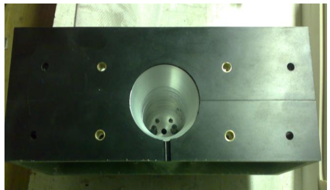
Fig. 3 Molds for the final propeller
