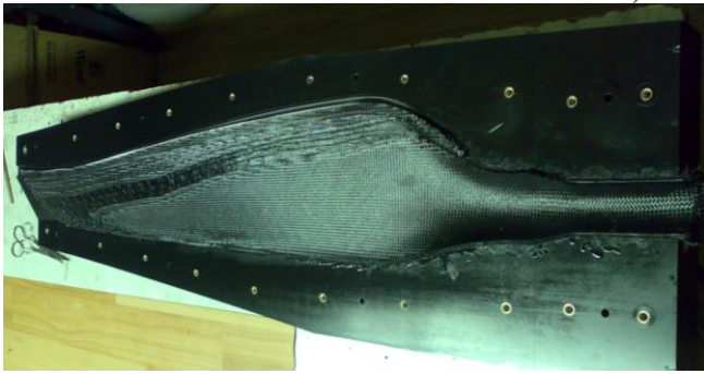
Fig. 4 Contact laminating layers of carbon fiber fabric
