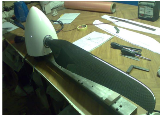
Fig. 7 The propeller blades after their assembling with the propeller head Woodcomp Ltd. labeled SR 3000/2W
