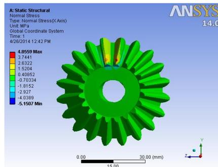
**Fig 29: Bevel gear on Top Normal Stress**
