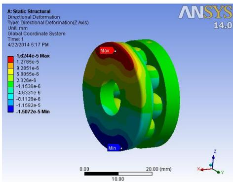
Fig 32: Ball Bearing Deformation
