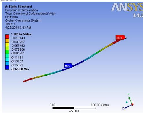
Fig 34: Deformation of Telescopic Shaft
