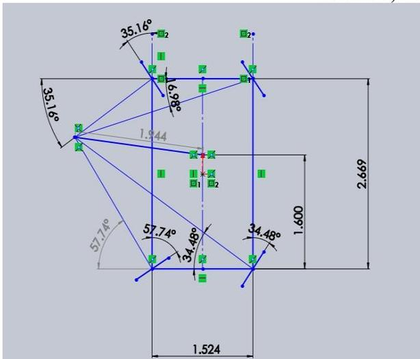
Fig 24: Turning Circle Radius drafted in SOLIDWORKS
