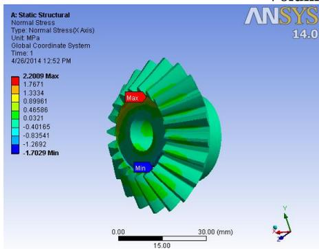
Fig 31: Bevel Side Normal Stress (Bending)
