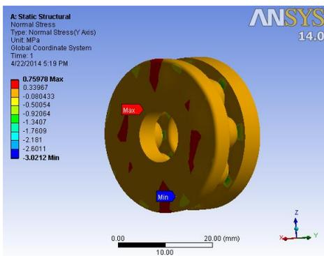
Fig 33: Ball Bearing Normal Stress
