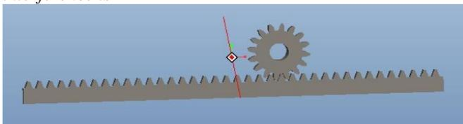
Fig 20: Rack and Pinion Assembly
