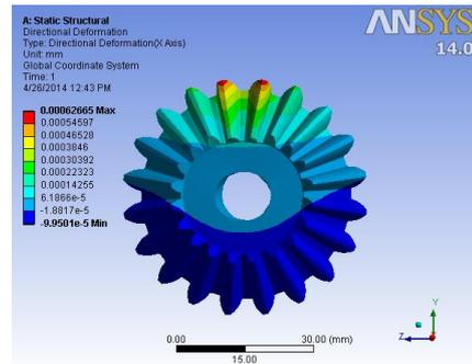
**Fig 28: Bevel Gear on top deformation**
