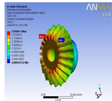
**Fig 30: Bevel Gear Side Deformation**
