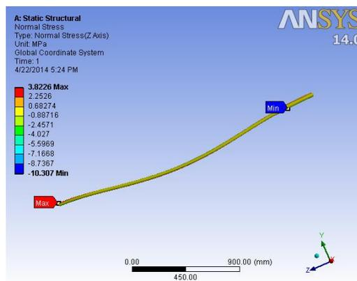
Fig 35: Normal Stress in Telescopic Shaft
