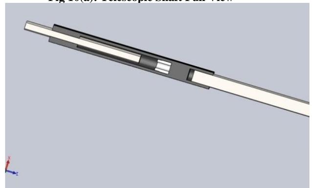
Fig 10(b): Telescopic Shaft Front Sectional View
