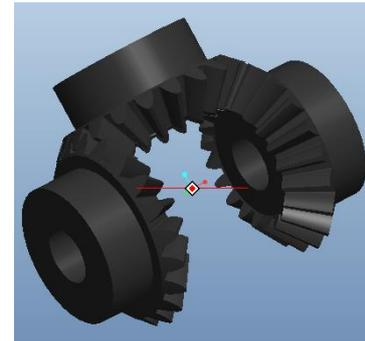
Fig 9: Bevel Gears
