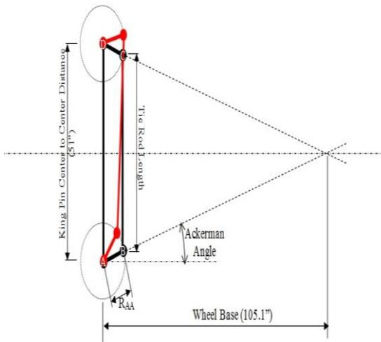
Fig 14: Ackerman Steering Mechanism
