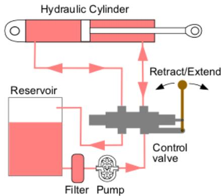
Fig 11: Hydraulic Circuit Directional Control
