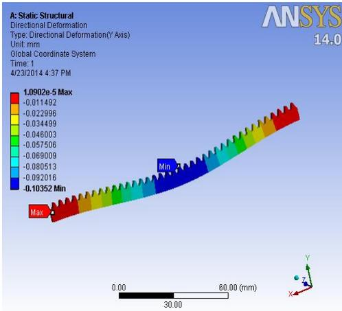
Fig 38: Rack Deformation
