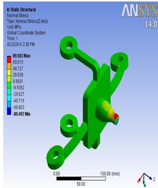
Fig 41: Spindle Normal Stress
