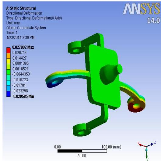
Fig 40: Spindle Directional Deformation
