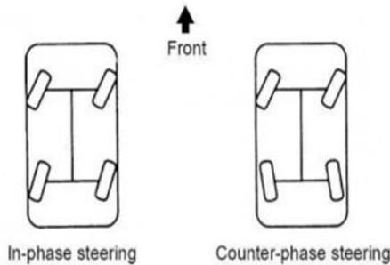
Fig 4: In-Phase and Counter-Phase Steering
