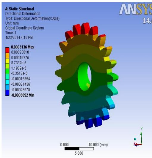
Fig 36: Pinion Deformation
