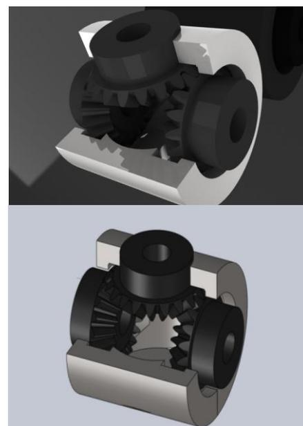
Fig 26: Bevel Gear Casing Assembly
