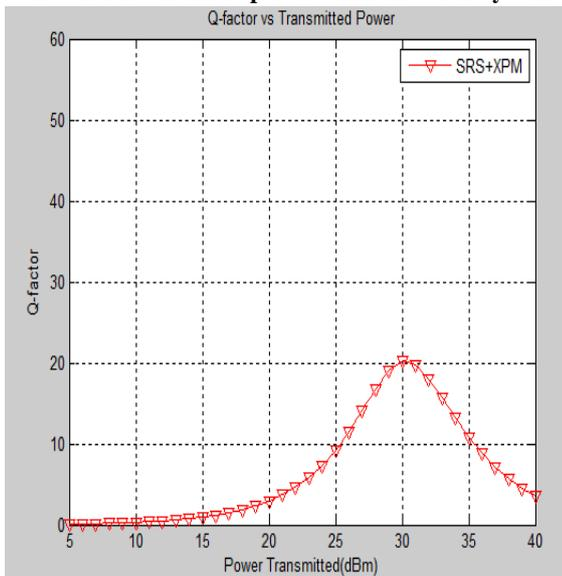
**Fig. 9 Transmitted Power Analysis SRS-XPM nonlinear effect for 16-channel optical communication System**
