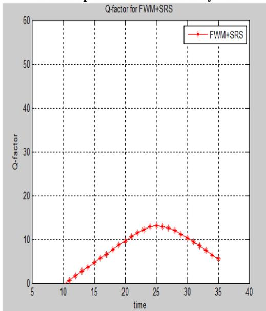
Fig. 3 Q-factor analysis FWM-SRS nonlinear effect for 16-channel optical communication System
