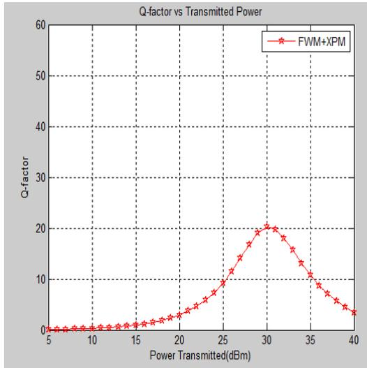
**Fig. 7 Transmitted Power Analysis FWM-XPM nonlinear effect for 16-channel optical communication System**
