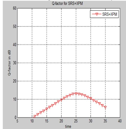
Fig. 4 Q-factor analysis SRS-XPM nonlinear effect for 16-channel optical communication System
