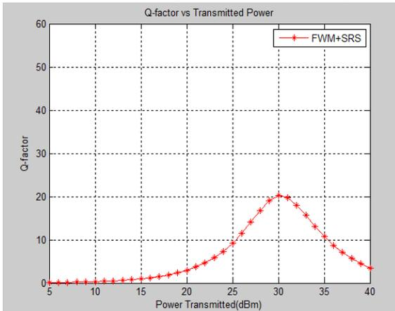
**Fig. 8 Transmitted Power Analysis FWM-SRS nonlinear effect for 16-channel optical communication System**
