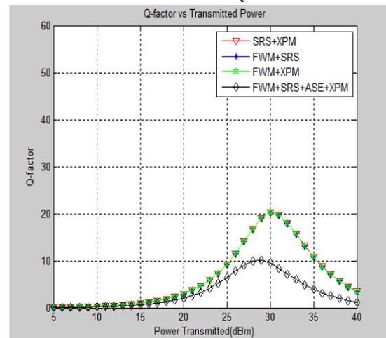
**Fig. 11 Combined Transmitted Power Analysis for different nonlinear and linear effect for 16-channel optical communication System**
