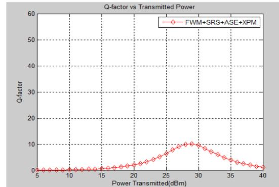
**Fig. 10 Transmitted Power Analysis FWM-SRS-ASE-XPM nonlinear and linear effect for 16-channel optical communication System**
