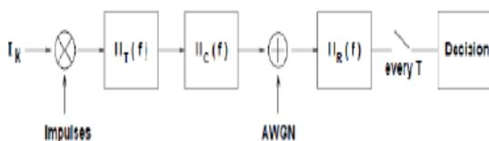
Fig. 5 ICI removal with equalizer
