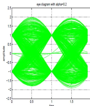
Fig 7 Eye Diagram with alpha=0.2
