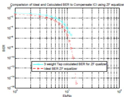
**Fig. 10 comparisons of Theoretical and Simulated Bit error probability to remove ICI using Zero Forcing (ZF) equalizer**
