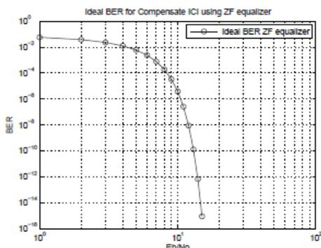
**Fig. 8 Theoretical Bit error probability to remove ICI using Zero Forcing (ZF) Equalizer**
