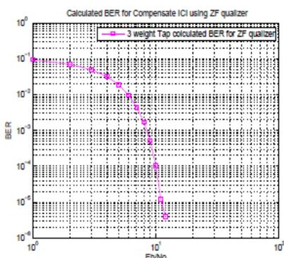
**Fig. 9 Simulated Bit error probability to remove ICI using Zero Forcing (ZF) equalizer**
