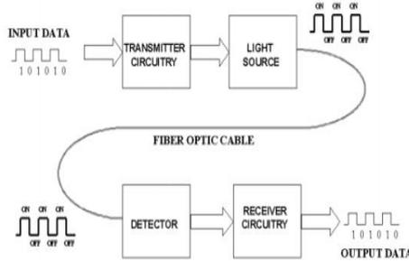
Fig. 1 Optical Communication System
