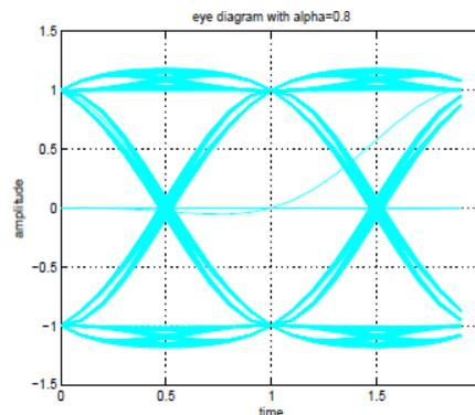
Fig. 6 Eye Diagram with alpha=0.8
