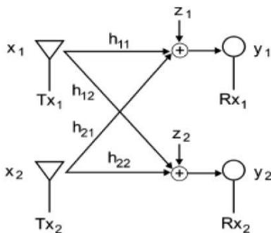
Fig. 2 Gaussian interference channel
