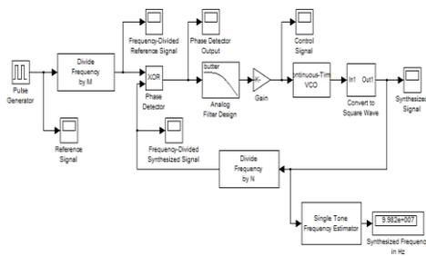
Fig. 7 Frequency synthesis of phase lock loop in the presence of noise
