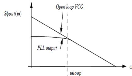
Fig. 5 Output phase noise spectrum with a noiseless input
