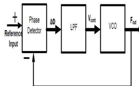
Fig. 1 block diagram of PLL
