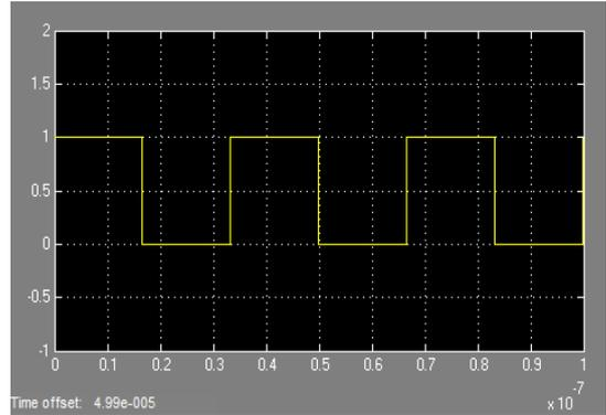
Fig. 8 Reference Signal to the input of PLL
