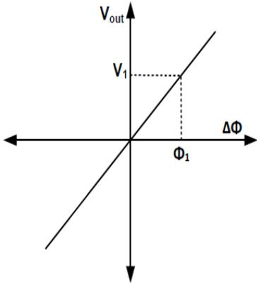
Fig. 2 Phase detector characteristics
