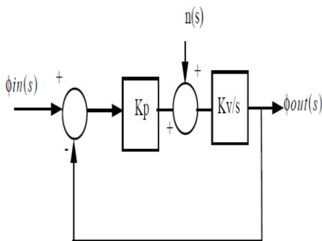
Fig. 4 Block diagram PLL with noise sources
