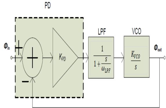
Fig. 3 Linear model of PLL
