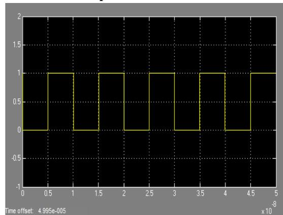
Fig. 10 Synthesis signal of the frequency synthesiser in the presence of phase noise
