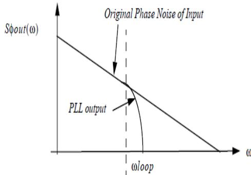
Fig. 6 Output phase noise spectrum with a noise less VCO
