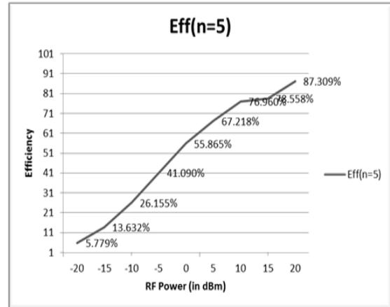
Fig. 9 a 5 stages (value of 'n') voltage doubler circuit for Efficiency (in %) with reference to the Received RF power.
