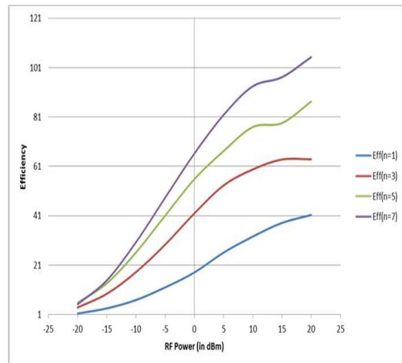
Fig. 11 stages (value of 'n') voltage doubler circuit for Efficiency (in %) with reference to the Received RF power
