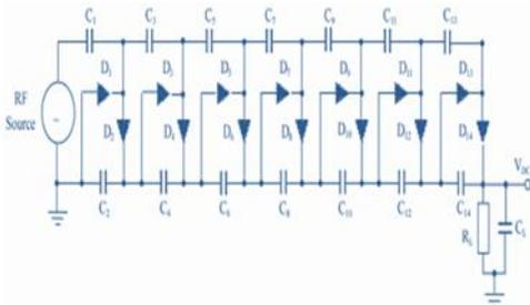
Fig. 4 Multistage Voltage Multiplier
