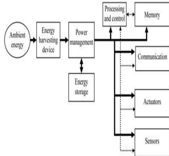
Fig. 2 WSN architecture with Energy Harvester circuit
