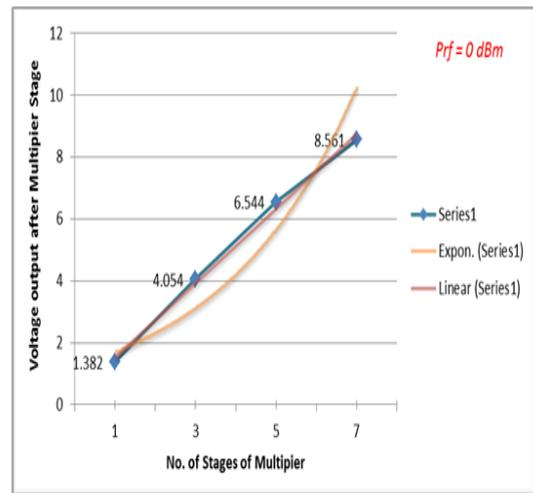
Fig.5 Voltage Multiplier o/p vs no. of stages
