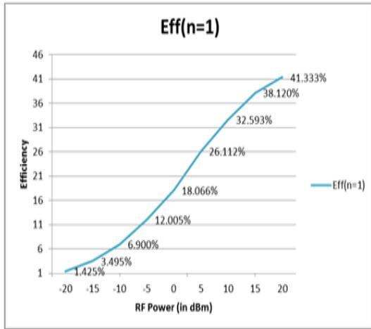
Fig.7 a 1stages (value of 'n') voltage doubler circuit for Efficiency (in %) with reference to the Received RF power
