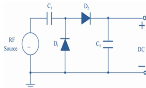
Fig. 3 Multiplier Circuit
