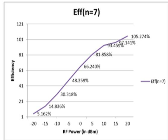
Fig. 10 a 5 stages (value of 'n') voltage doubler circuit for Efficiency (in %) with reference to the Received RF power.
