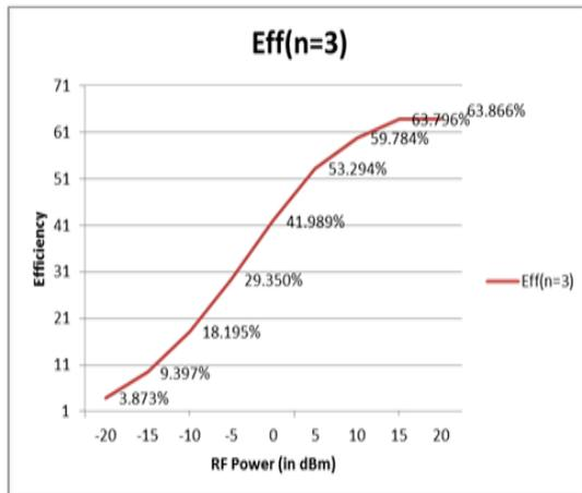
Fig.8 a 3 stages (value of 'n') voltage doubler circuit for Efficiency (in %) with reference to the Received RF power
