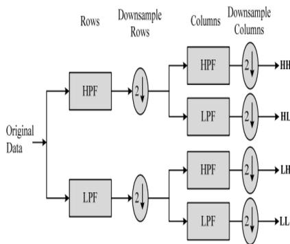
Fig. 2 Block diagram of 2-D forward DWT
