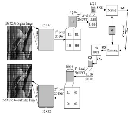
Fig. 5 Block diagram of the DWT decomposition
