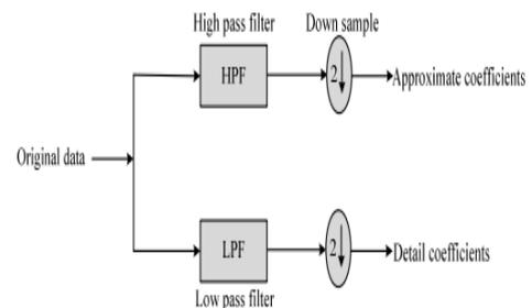
Fig.1 Block diagram of 1-D forward DWT
