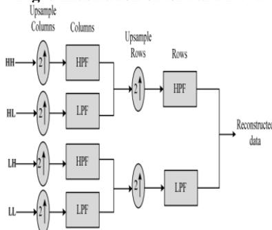
Fig. 4 Block diagram of 2 dimensional inverse DWT
