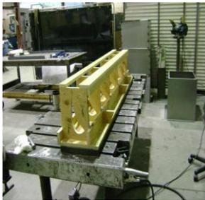
FIG 11: SLAT ASSEMBLY JIG
