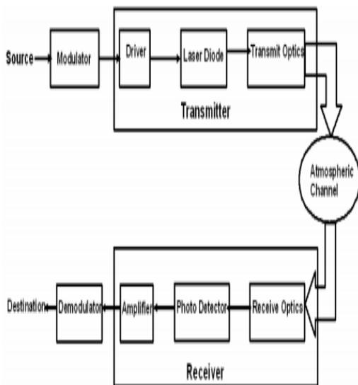
Fig. 1 Block diagram of FSO communication system
