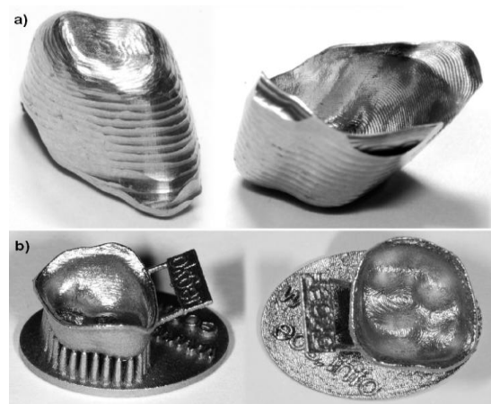
Fig. 6 Substructure of titanium crown: (a) using subtractive manufacturing technology with milling, (b) following additive laser sintering
