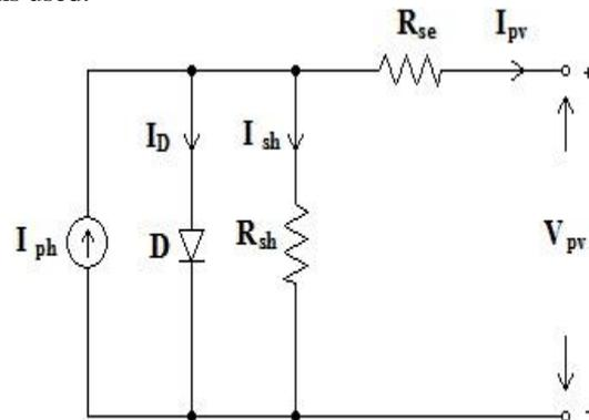
Fig.1. Equivalent circuit of SPV cell [6]
