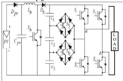
**Fig.2. Seven level inverter for PV systems [1]**
