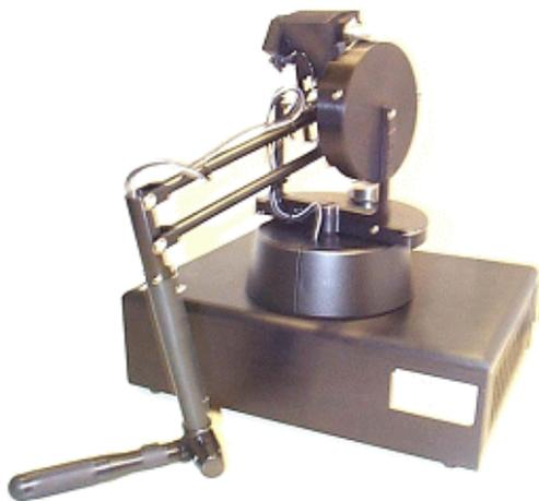
Fig 3 PHANToM - Haptic device
