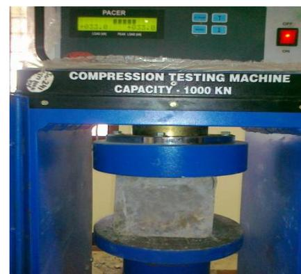
Fig. 2 Cube testing in CTM
