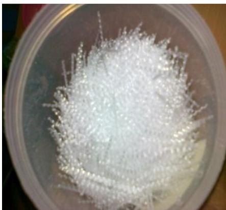
Fig. 1 Endura-600, Macro synthetic Poly Propylene fiber
