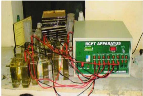
Fig. 6 RCPT Test set up
