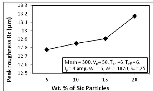
Fig. 13 Peak Roughness Rz(µm) Vs Wt. % of Sic Particles
