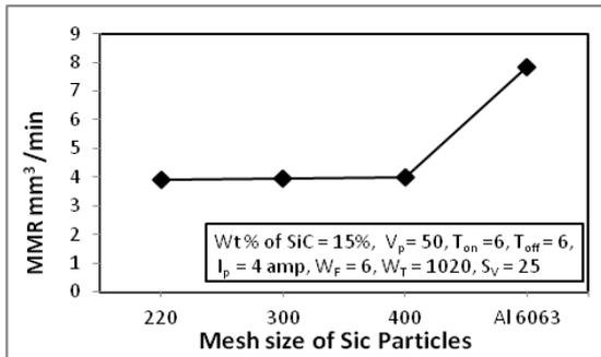
Fig. 6 MMR mm<sup>3</sup>/min Vs Mesh size of Sic Particles
