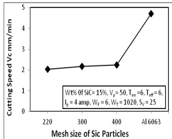
**Fig. 3 Cutting Speed  $V_c$  mm/min Vs Mesh size of Sic Particles**
