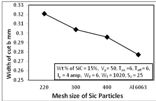
Fig. 5 Width of cut b mm Vs Mesh size of Sic Particles
