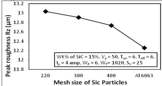
Fig. 7 Peak Roughness Rz(µm) Vs Mesh size of Sic Particles
