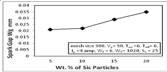
Fig. 10 Spark Gap Wg mm Vs Mesh size of Sic Particles
