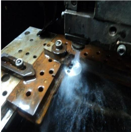
**Fig.2 Machined number of Cubes by WEDM**
