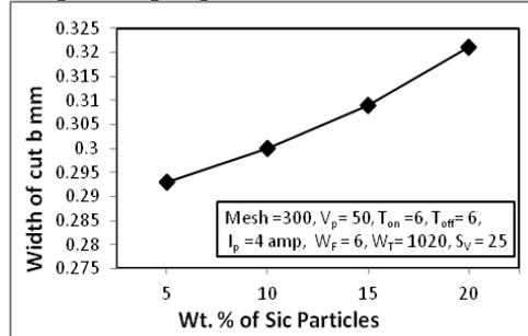
Fig. 11 Width of cut b mm Vs Wt. % of Sic Particles
