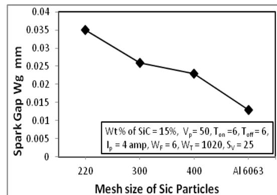
**Fig. 4 Spark Gap  $W_g$  mm Vs Mesh size of Sic Particles**
