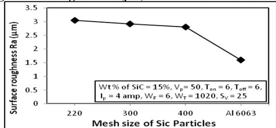
Fig. 8 Surface roughness Ra (µm) Vs Mesh size of Sic Particles
