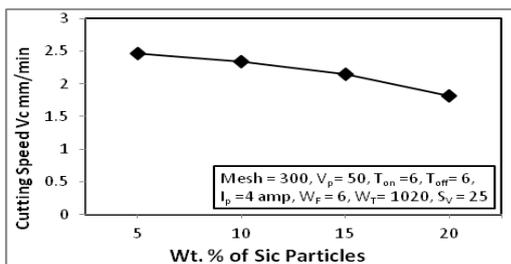
Fig. 9 Cutting Speed Vc mm/min Vs Wt. % of Sic Particles
