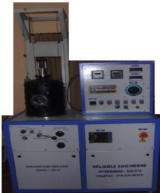
Fig.1. Thermal Evaporation Unit
