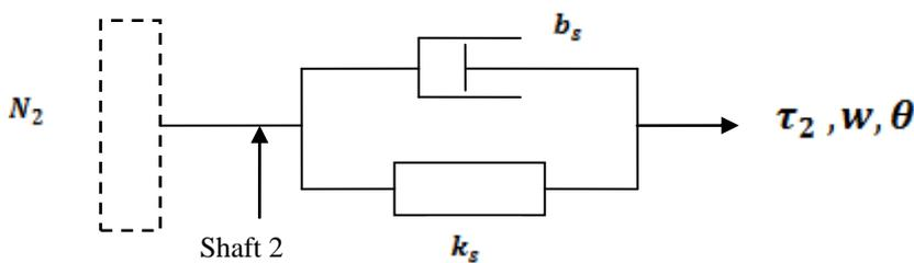
Fig. 6: Transmission Shaft linking the load and gear mechanism
