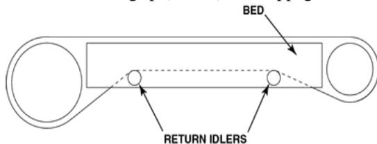
Fig. 3: Underneath belt supported by Return Idlers [1]
