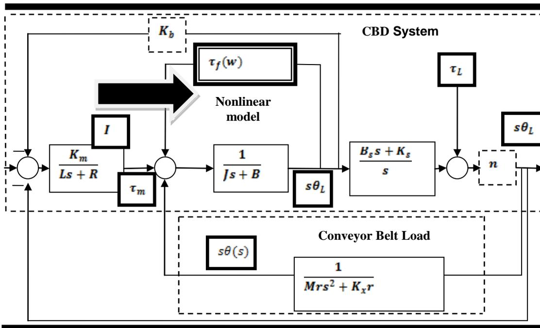
Fig. 9: Block Diagram for the Conveyor model
