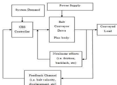
Fig. 1: Schematic Block Diagram of a Conveyor System
