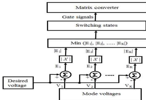
Fig. 3: Control strategy of switching pulse generation [8]
