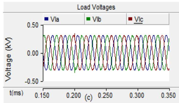
**Fig. 8: Simulation results of DVR with matrix converter under unbalanced swell (a) Source voltages (b) Injecting voltages and (c) Load voltages**
