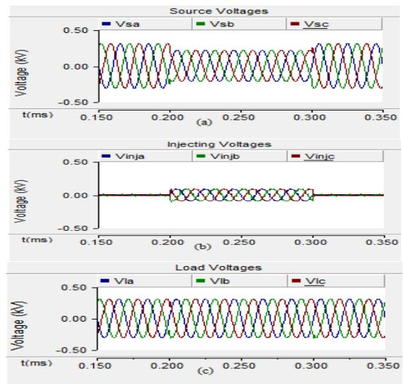
Fig. 5: Simulation results of DVR with matrix converter under balanced sag (a) Source voltages (b) Injecting voltages and (c) Load voltages
