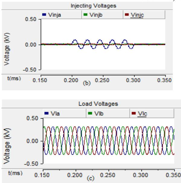
**Fig. 6: Simulation results of DVR with matrix converter under unbalanced sag (a) Source voltages (b) Injecting voltages and (c) Load voltages**
