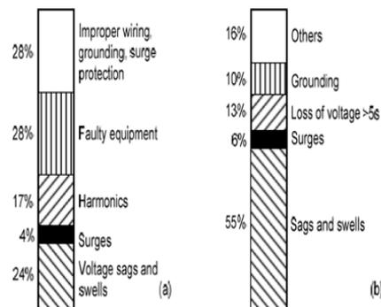
Fig. 1: Basic disturbances (a) at customer side (b) at utility side [1]
