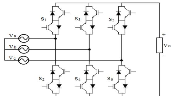
Fig. 2: Switching Arrangement in Matrix Converter [8]
