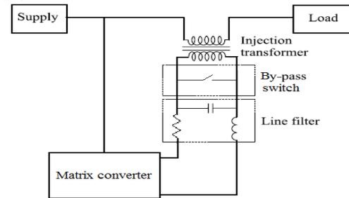
Fig. 1: Schematic diagram of DVR with matrix converter [5]
