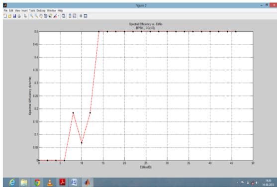
Fig 5: Plot of Spectral Efficiency for BPSK-WIMAX
