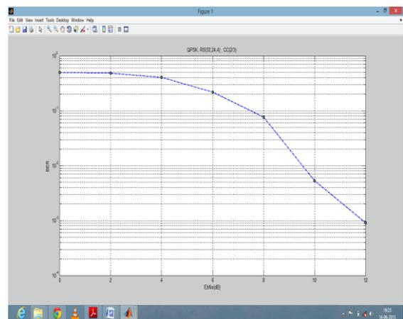
Fig 2: Plot of BER against Eb /No For QPSK-WIMAX.
