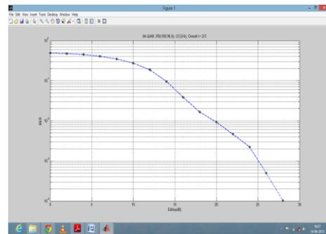
Fig 8: Plot the BER against Eb /No for QAM 64-WIMAX.
