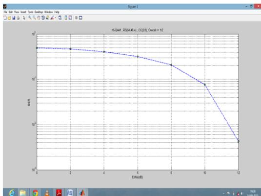
Fig 6: Plot the BER against Eb /No for QAM 16-WIMAX.
