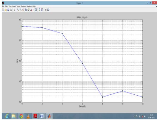
Fig 4: Plot of BER against Eb /No for BPSK-WIMAX.
