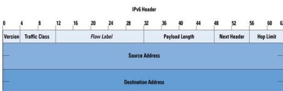
Fig 2: IPv6 and IPv6 Header Format
