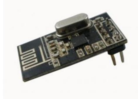
Fig. 6 2.4 Ghz RF Transceiver
