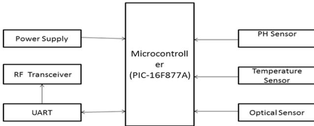
Fig. 1 Transmitter Block Diagram
