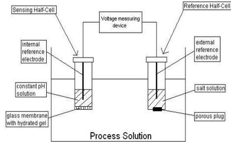
Fig. 3 pH Sensor Operation
