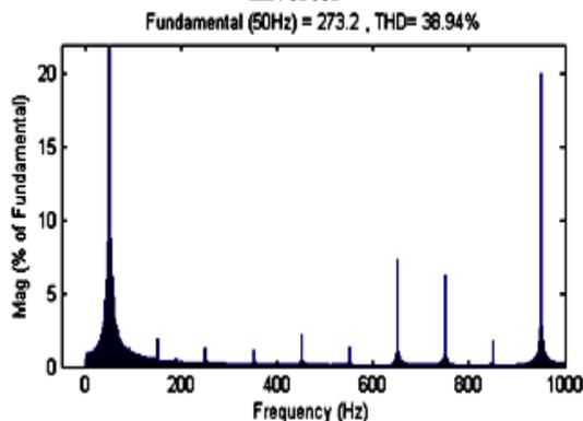
Fig.16: FFT Analysis of Conventional Cascaded Inverter
