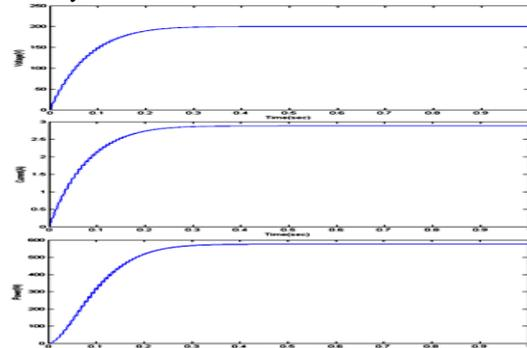
Fig.13: Output Voltage, Current and Power of Multistring PV Boost Converter
