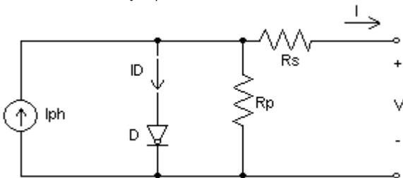
Fig.7: Equivalent Circuit for the Solar Module [19]
