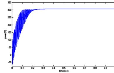
Fig.12: Maximum Power Obtained From MPPT
