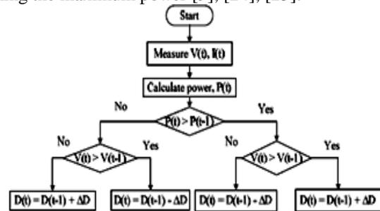
Fig.8: Flowchart for P & O algorithm [9]
