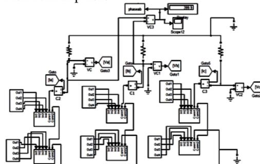
Fig.14: Simulink Model of Conventional Cascaded Inverter with Multi-String PV System
