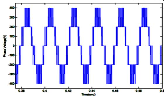
Fig.15: Output Phase Voltage of Conventional Cascaded Inverter
