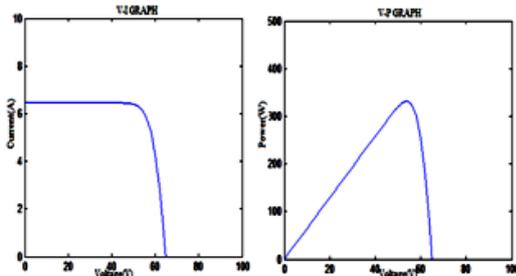
Fig.11: V-P and V-I output characteristics of PV module at T=25°C and s=1kW/m<sup>2</sup>
