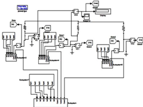
Fig.17: Simulink Model of Proposed Cascaded Inverter with Multi-String PV System
