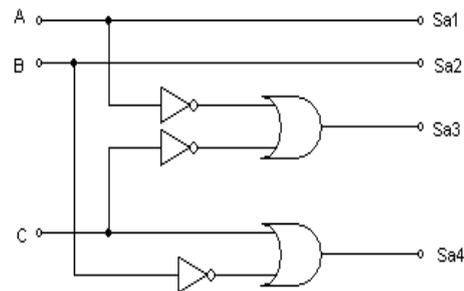
Fig.6: Switches Logic Control Schematics [14]
