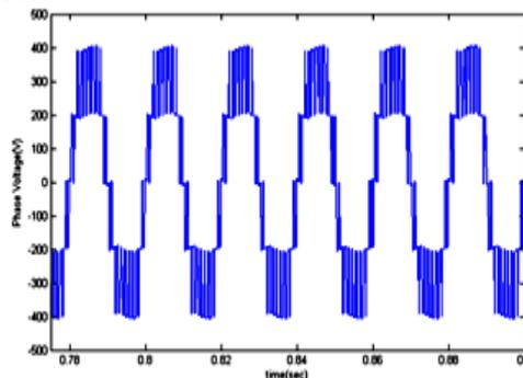
Fig.18: Output Phase Voltage of Proposed Cascaded Inverter System
