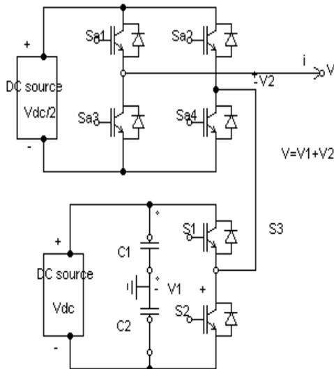
Fig.3: Single Phase Structure of Proposed Inverter [28]
