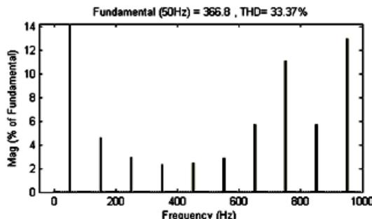
Fig.19: FFT Analysis of Proposed Cascaded Inverter
