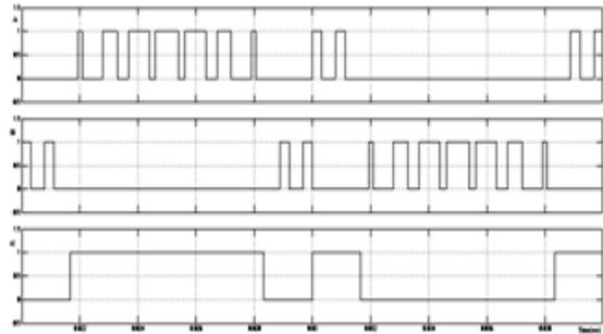
Fig.5: PWM Pulses of Single Phase Bridge Inverter
