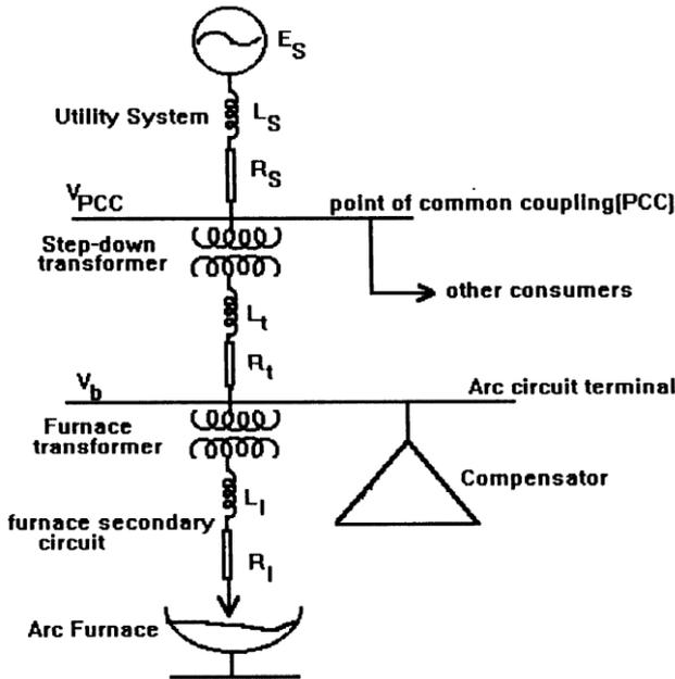
Fig. 1. Single phase supply network diagram of an electric arc furnace
