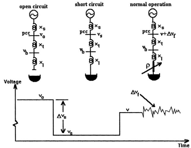
Fig. 3. Voltage changes due to operating state of an electric arc furnace
