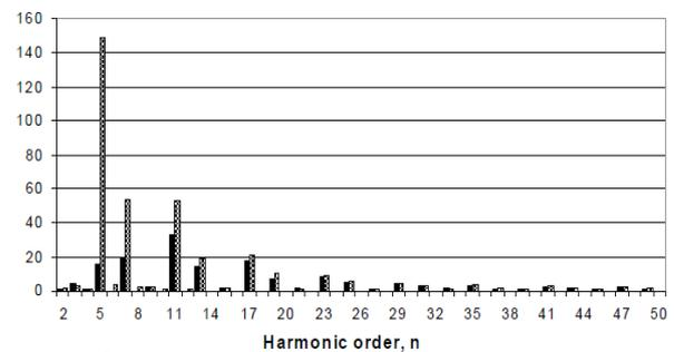
Fig.11. Current distortion on nonlinear load when breaker closed
