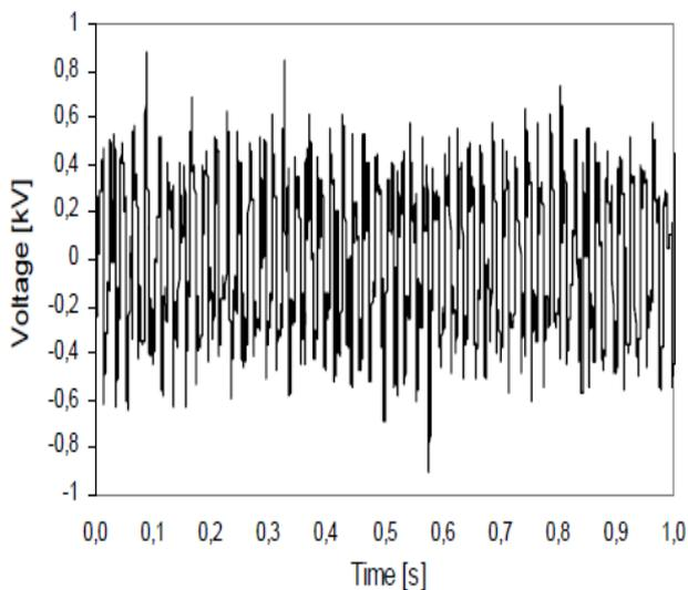
Fig.8. Voltage waveform at the Arc Furnace
