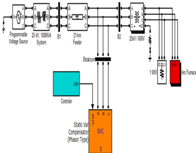
Fig.7. simulink model of under study system
