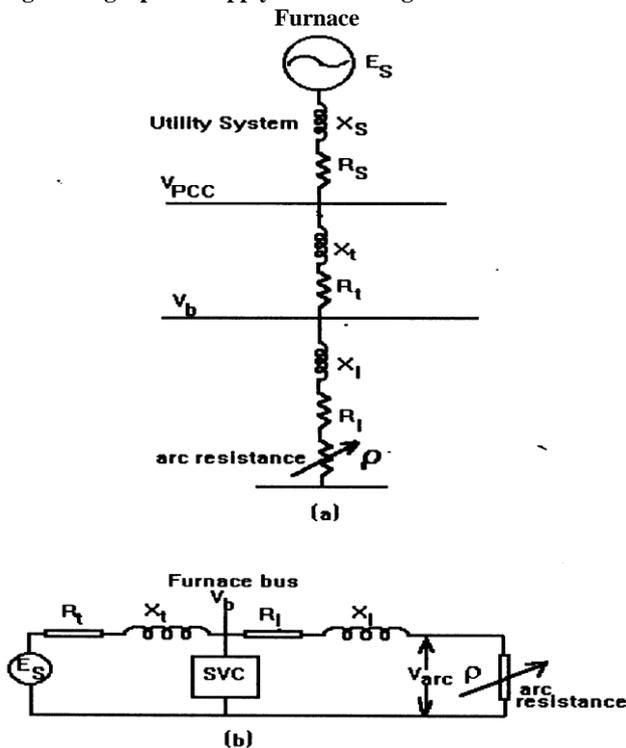
Fig. 2. Derivation of single-phase equivalent circuit for estimating furnace operating characteristics
