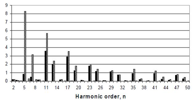
Fig.10. Voltage distortion on nonlinear load when breaker closed
