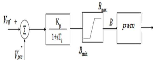
Fig.4. Block diagram of SVC PI controller.
