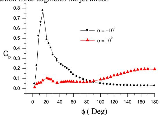
Fig 6 Circumferential Pressure Distribution In A Plane Passing Through Centre Of Jet At ( $X/D = 1.236$ ),  $M_\infty = 8.1$ ,  $A = 5^\circ$ ,  $JPR = 1100$ , Jet Mass Flow
