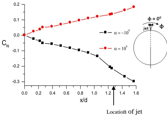
Fig-7 Longitudinal Normal Force Coefficient Distribution On Leeward Surface ( $\Phi = 0^\circ$ ) With Jet-On Condition At  $M_\infty = 8.1$ ,  $JPR = 1100$ . Altitude = 35 Km
