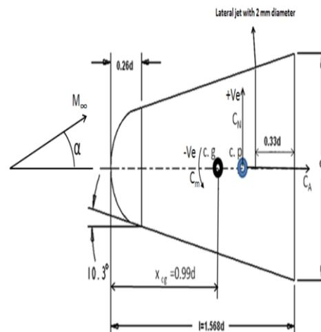
Fig 1 Schematic View of Model with Sign Convection Used For Normal Force and Pitching Moment
