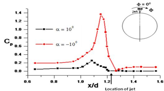
Fig 5 Longitudinal Pressure Distribution In Jet Interaction Area  $X/D = (0.6 \text{ To } 1.568)$
