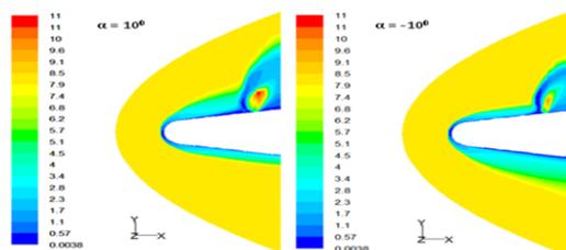
Fig 4 Mach Contours At  $A = 10^\circ$  and  $A = -10^\circ$
