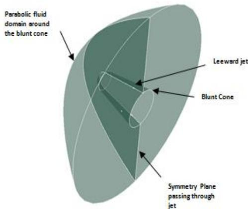
Fig 2 Fluid Domain around Vehicle
