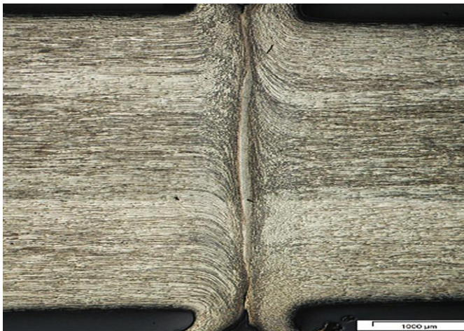
Fig. 7. The shape of the flash under the rotation friction welding process. [16]
