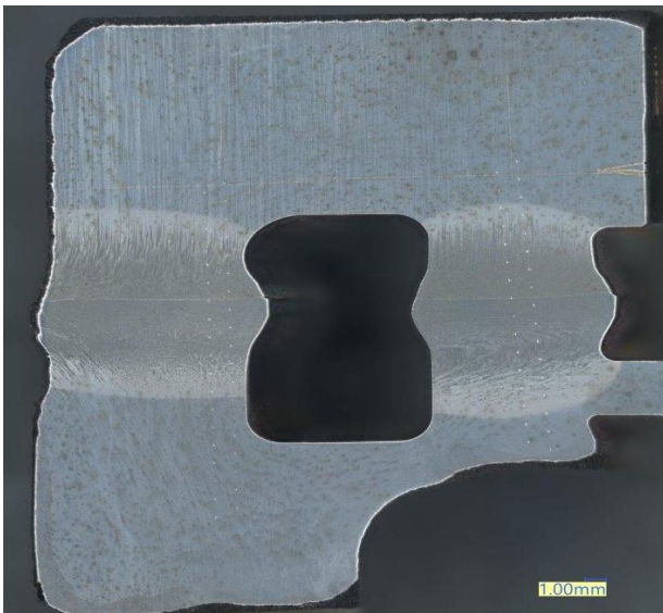
Fig. 17: View of the tested welded joint, with traces left by the hardness measurement.
