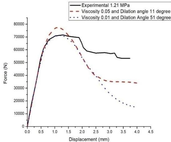
**Fig. 9. Force Displacement Curve for Selected Parameters from Sensitivity Analysis for a Pre-Compression Load of 1.21 MPa**
