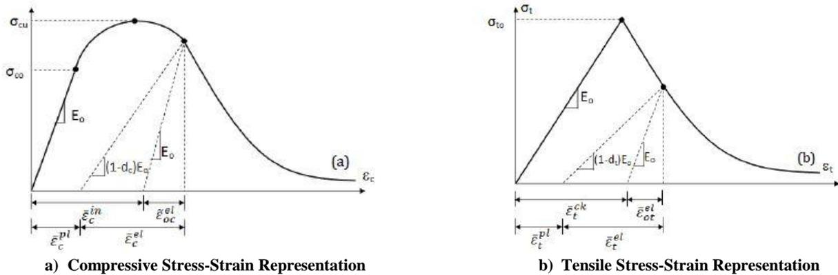
Fig. 2. Stress-Strain Representation of Concrete or any quasi-brittle material [14]
