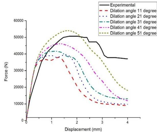
**Fig. 7. Sensitivity Analysis with the variation of dilation angle for Viscosity Coefficient of 0.01**
