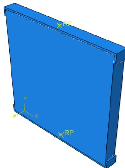
Fig. 4. Homogenized Masonry Panel with Steel Beam at Top and Bottom
