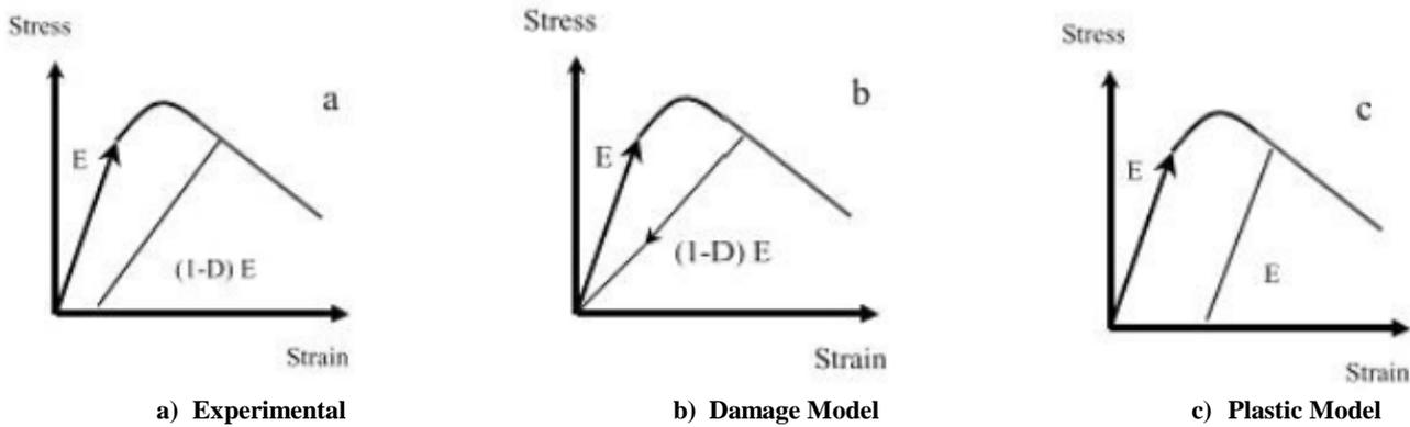
Fig. 1. Loading-Unloading Behavior, Experimental and Simulated Behavior [13]
