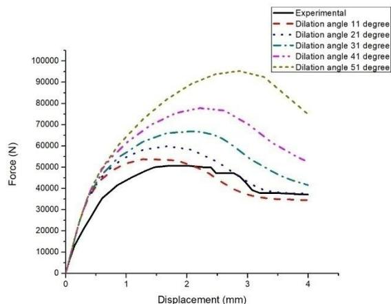
**Fig. 8. Sensitivity Analysis with the variation of dilation angle for Viscosity Coefficient of 0.05**
