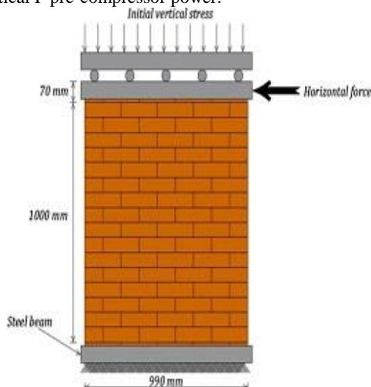
Fig. 3. Experimental Wall used for Validation of Proposed Method [15]
