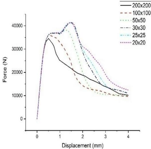
**Fig. 5. Force vs Displacement Curve for Various Mesh Size for Considered Masonry Wall for a Pre-compression load of 0.3 MPa**
