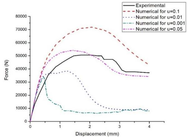
**Fig. 6. Sensitivity Analysis with variation of viscosity parameter for Force displacement relation**
