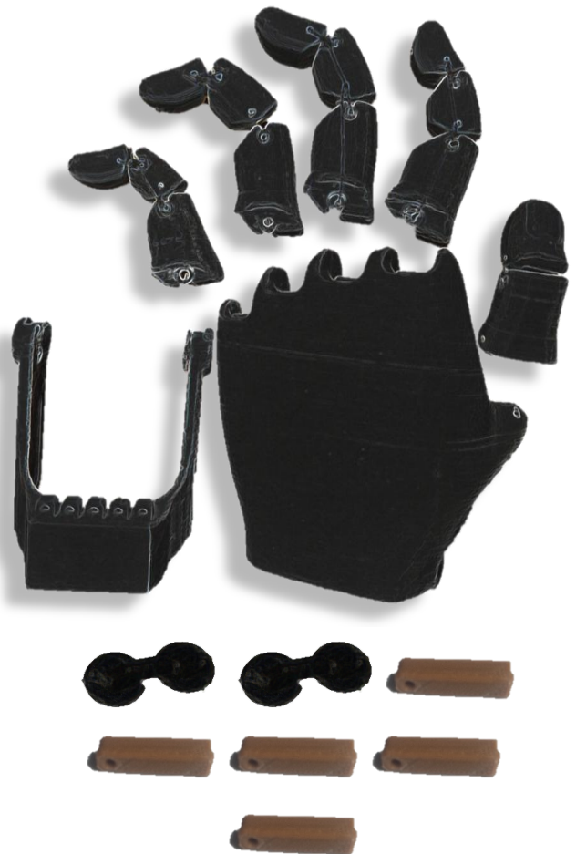
Fig.10.3D-Printed parts (components) of the prosthetic limb.
