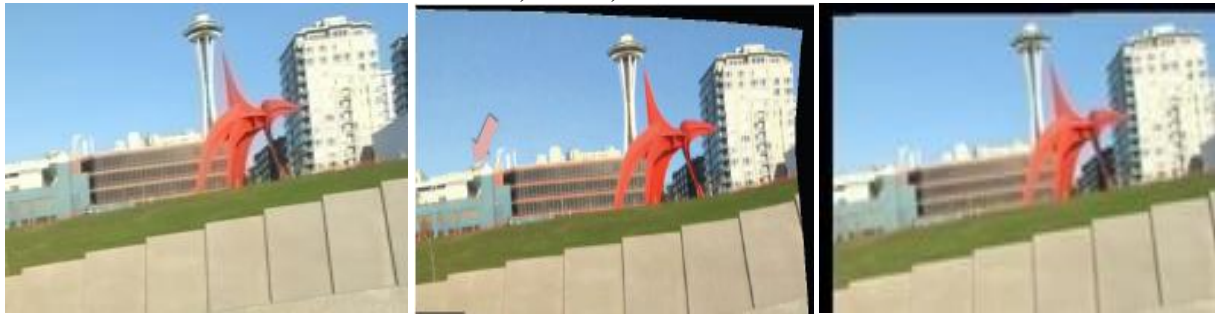
Fig. 7. Comparison of Global vector stabilization a) 75 th Frame b) Result of Lei Zhang, et al [1] c) result of estimation with proposed truncated frame error method
