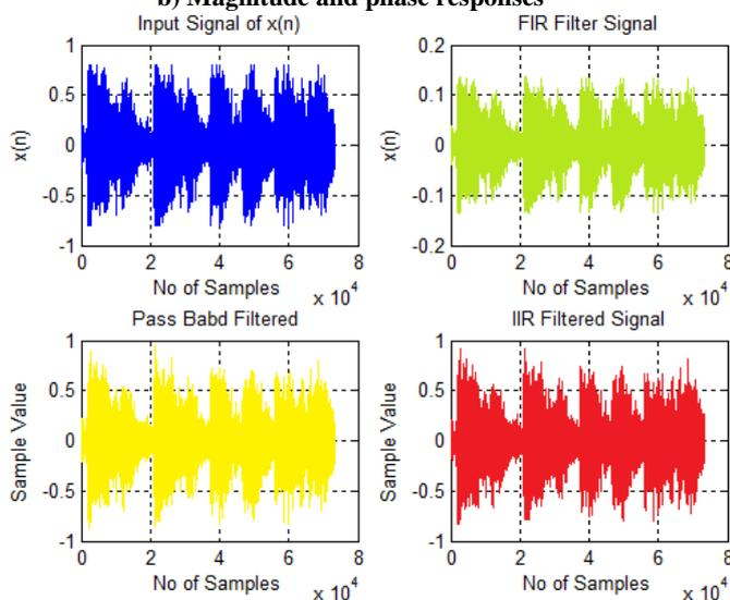
**Fig.8. Comparison of the Filtering performance FIR Vs IIR**
