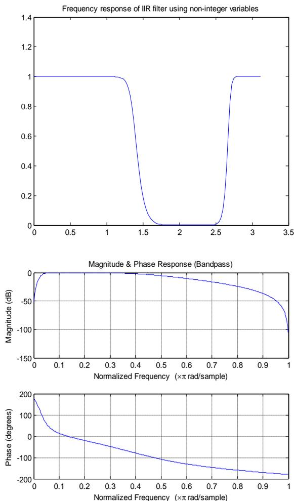
**Fig.7. Two step IIR Filter Responses, a) frequency response of the proposed IIR filter with optimum parameter tuning. b) Magnitude and phase responses**
