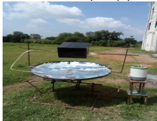
Fig.4. Previous experimental model of dish collector and receiver system.
