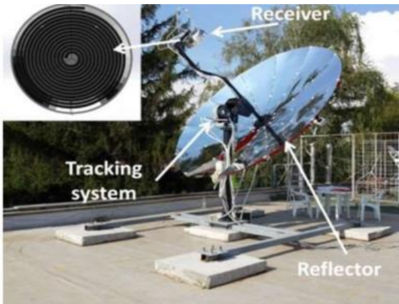
Fig.2. Parabolic dish collector system
