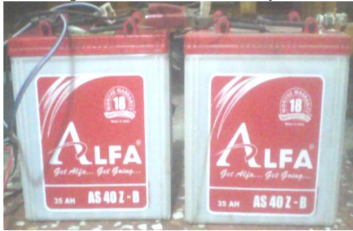
Fig 8: Lead acid battery
