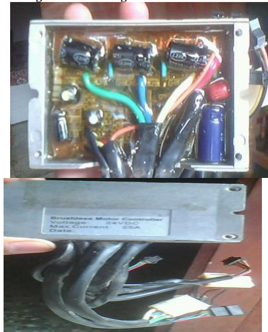
Fig 12: Hub motor controller
