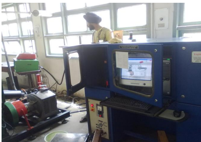
Fig.1 Computerized Variable Compression Ratio Multi-Fuel Engine Test Rig
