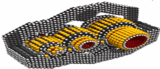
With 15,342 atoms, this parallel-shaft speed reducer gear is one of the largest nano mechanical devices ever modeled in atomic detail.
