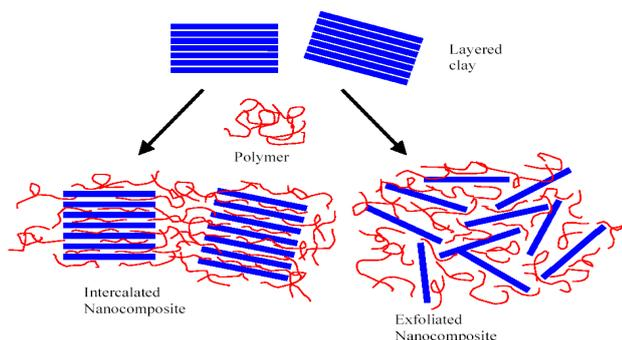
**Fig 6 Polymer-Clay Nano Composites**
