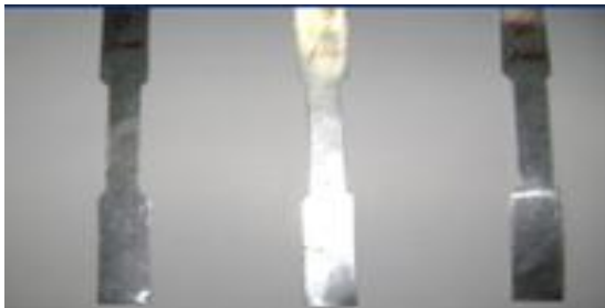
Fig. 2 Tensile test Pieces of AA 1100
