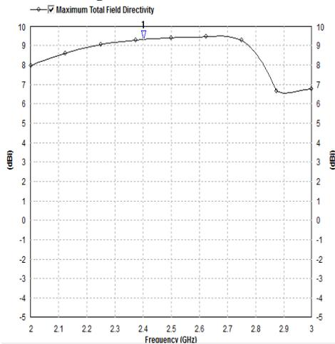
**Fig.5. Directivity of Antenna**
