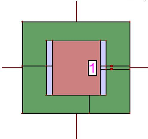
**Fig.2. Designed Stacked Square Patch Antenna**
