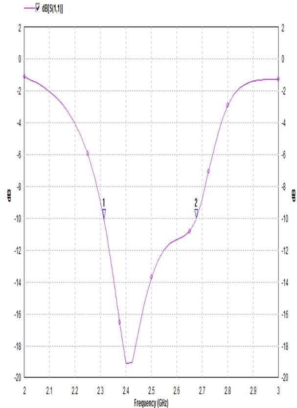
**Fig.3. Return loss of antenna**
