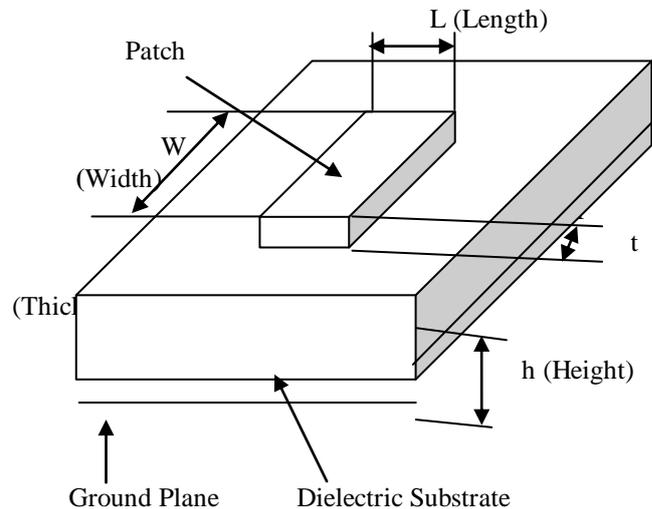
Fig.1. Microstrip Patch Antenna
