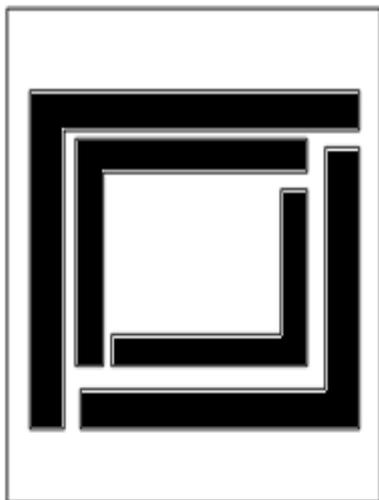
Fig. 3:- Second Order Shape of L- Shaped Meandered Quasi Fractal Antenna
