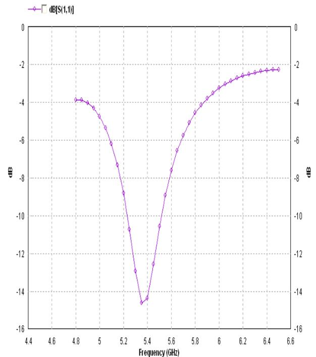
Fig. 5:- Return Loss for Base Shape
