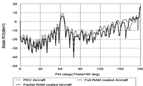
**Fig. 4. Bistatic RCS of aircraft at 1 GHz.**
