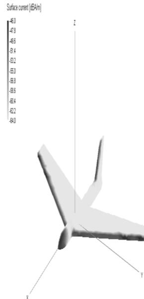
**Fig. 7(A). Current Density on A PEC Aircraft & Fig.7 (B). Current Density On A RAM Coated Aircraft.**
