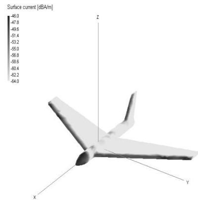
**Fig. 6. Bistatic RCS of aircraft at 10 GHz.**
