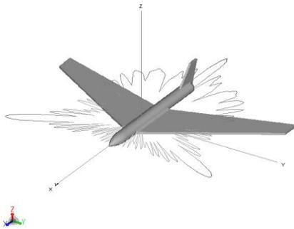
Fig. 1. Plane Wave Incidence at the Nose of an Aircraft and RCS Pattern In the  $\phi$ -Plane.
