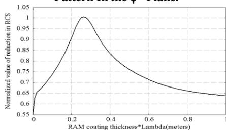
Fig. 2. Normalized value of reduction in Bistatic RCS of aircraft with RAM thickness (expressed in terms of wavelength) at 1GHz.
