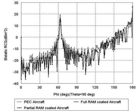
**Fig. 5. Bistatic RCS of aircraft at 3 GHz.**
