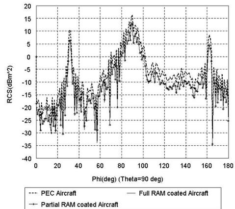
Fig. 3. Monostatic RCS of aircraft at 1 GHz.
