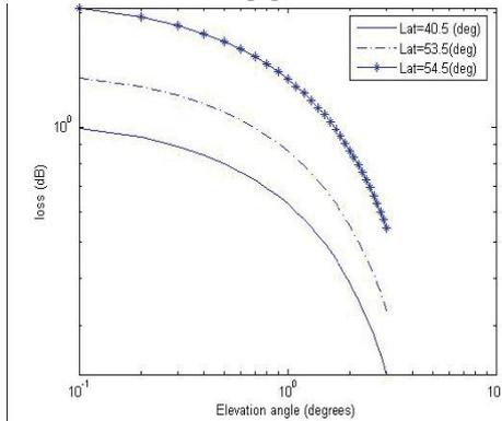
**Fig 6: Loss With Respect To Elevation Angle as a Function of Latitude [9].**
