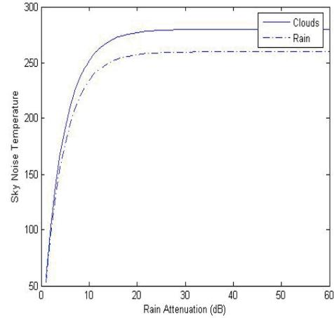
**Fig 5: Sky Noise Temperature As Seen By the Antenna [8].**
