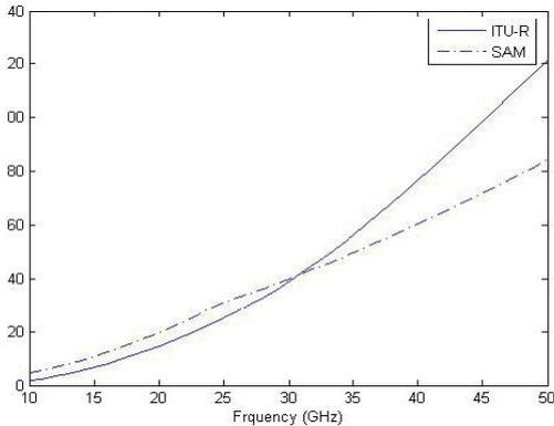
**Fig 3: Rain Attenuation As Determined By ITU-R Model And Simple Attenuation Model (SAM) At Frequencies Above 10 GHz [7].**
